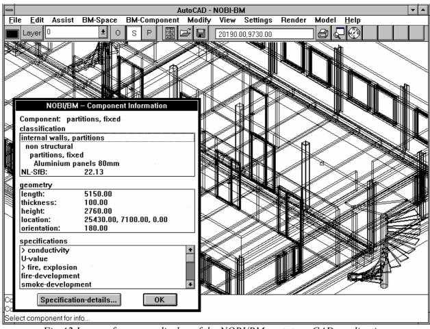
Fig.A2 Image of a screen-display of the NOBI/BM prototype CAD-application.
