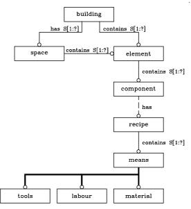
ponents is described in recipes that *Fig.2 Interpretation of BBB cost-engineering model.* contain the composition of components out of project-independent 'means'. An interpretation of the BBB model is given in EXPRESS-G, see figure 2.
